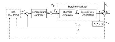
• Objective for batch k: tracking of supersaturation profile  $\overline{\mathbf{S}}_k$ .
