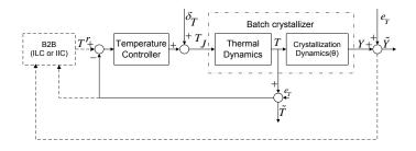
Objective for batch k: tracking of supersaturation profile Sk.
